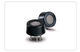
The KGS 102 is an  $S_nO_2$  semiconductor gas sensor and is used in gas detection, air cleaning system, auto-ventilation system, microwave oven, etc. In a clean atmosphere, the resistance of the sensor is high. However, with the increase of water vapor or gas concentration in the atmosphere, the resistance decreases. The KGS 102 gas sensor features high stability level against air flow, superb response time and excellent durability.
